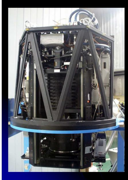
Size: 1035 mm x 960 mm *\phi* Weight: 295 kg Power: 420 W F: 1.86 FOV: 30' *\phi* CCD: MIT/LL CCID20 Format: 4096x2048 per CCD # of CCD: 10 (2 x 5) Filter: B,V,Rc,Ic,g',r',I',z'
